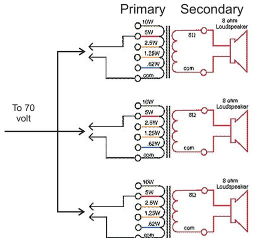
These 8 Ohm Loudspeakers with 70 Volt matching transformer (Fourjay ST5-CR8) are daisy chained using 18ga stranded twisted pair. Choose the 1 watt tap on the matching transformer for most applications.
